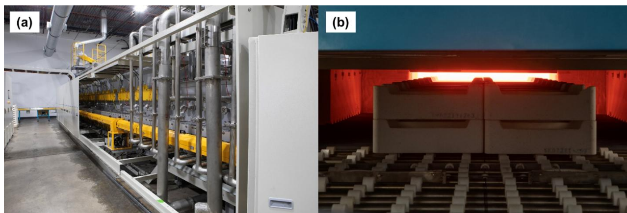
Figure 3. Photograph of the Dryve 13.5 m long RHK with insulating covers removed showing gas handling system and roller/heater covers (a) and sagger arrangement within the RHK entering the kiln ‘hot zone’ (b).
